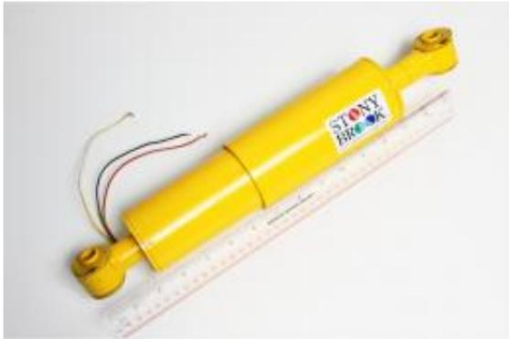
The shock absorber harvests energy from vibrations experienced by a vehicle's suspension system into electricity that can charge the battery and power vehicle electronics. Image credit: Lei Zuo
